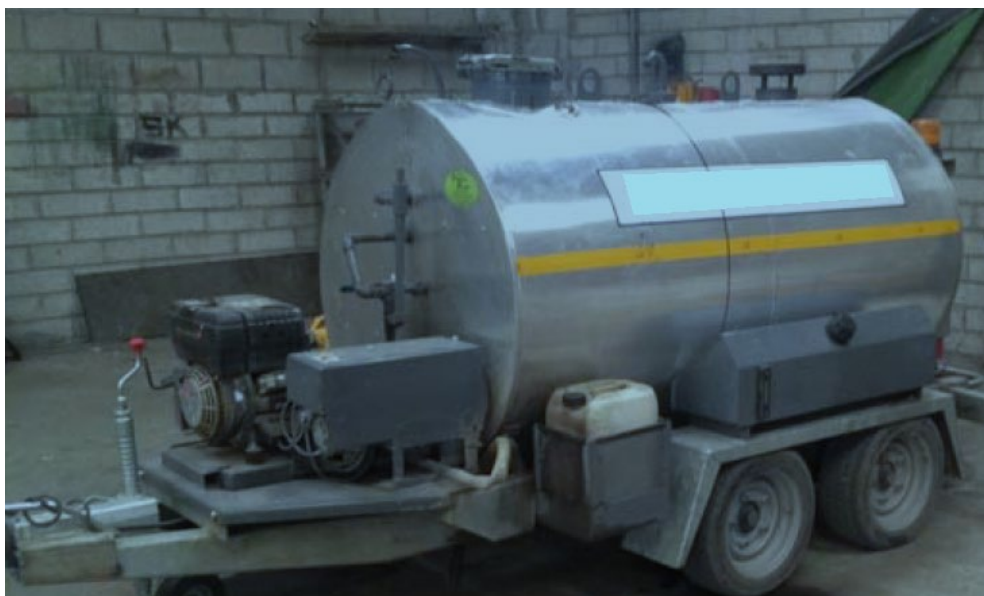
Figure 3-16: Towable Sprayer for Temporary Reinstatement
